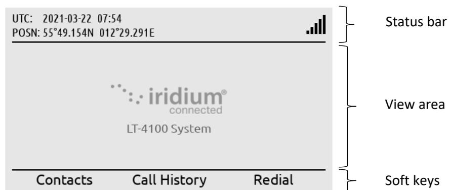
Figure 36: LT-4110 Control Unit - UI display sections
