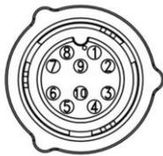
Figure 27: AUX cable pin out
