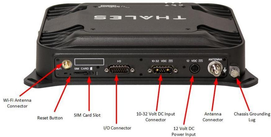
*Figure 1-5 Below Deck Unit (BDU) Back Panel Detail*
