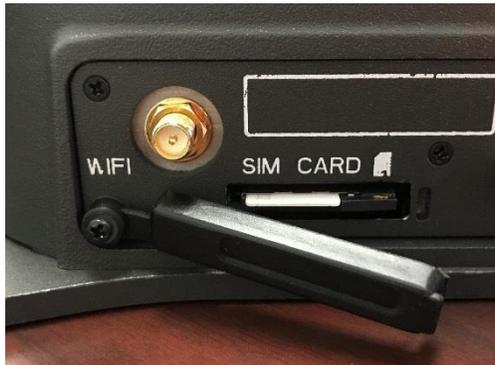
*Figure 2-12 SIM Card with Cover Opened*
