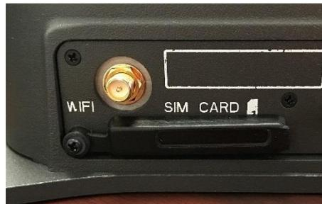
*Figure 2-14 Secure the SIM Card Cover*
