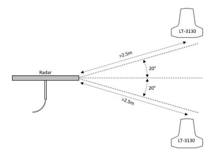
**IMPORTANT**: Failing to obey the specified installation conditions will void the warranty. However, depending on the specific radar frequency and power level, the separation distance between the radar and the Antenna Unit may be reduced, with no impact on the antenna performance. The performance of the Antenna Unit should be validated when the system is installed.
