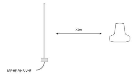
The Antenna Unit must be installed with a 360° clear view of the sky. However, minor obstructions such as a mast will not degrade the antenna performance severely, if a separation distance larger than 15 times the diameter of the obstruction is kept.
