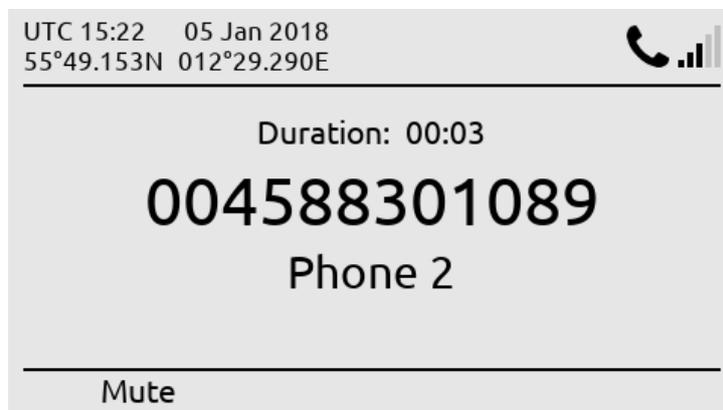
Figure 29: LT-3110 Control Unit – voice call successfully connected.
