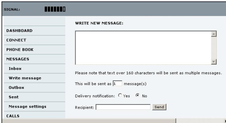
3. Type in the message in the **Write new message** field. If the message text is too long for one SMS, the message is sent as two or more SMS messages. The field below the message field shows the number of SMS messages used to send the message.
