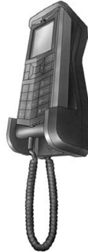
When the IP handset is used with the terminal, it communicates using IP between the handset and the terminal. However, on the BGAN network side of the terminal, calls may be transmitted as either circuit-switched or VoIP calls.
