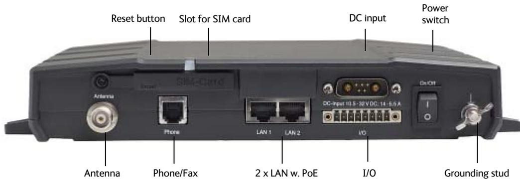
**Note** In this manual, the connector marked **Phone** on the connector panel is referred to as **Phone/Fax**.
