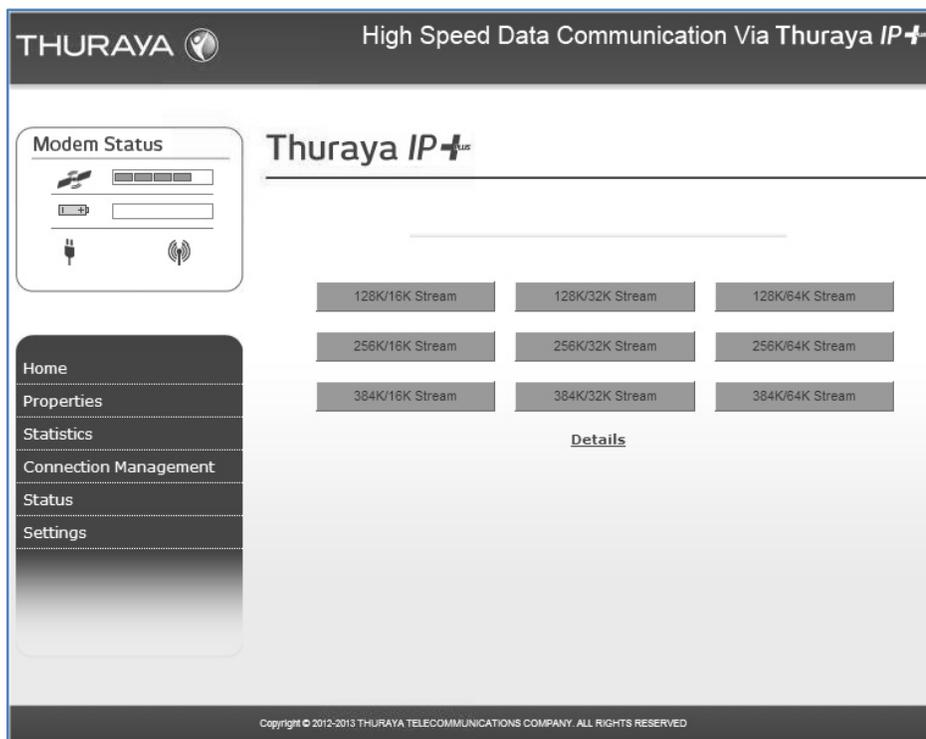
Accessible from the Main Menu, the **Connection Management Screen** allows you to select from nine Quality of Service (QoS) quick connect buttons. Each button can be customized using the **Details** link on the Connection Management Screen. The customization parameters for each button are as follows:
