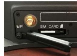
Install SIM card from Air-time provider as below. Insert card with contacts down as shown until it clicks into place. Be sure to engage the lock for the SIM Card and secure the SIM Cover once the SIM Card has been locked into place.
