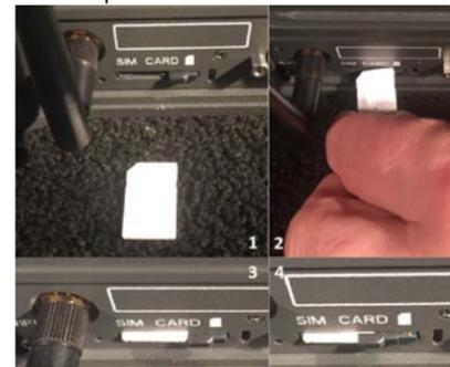
Installing SIM card and engaging the lock
