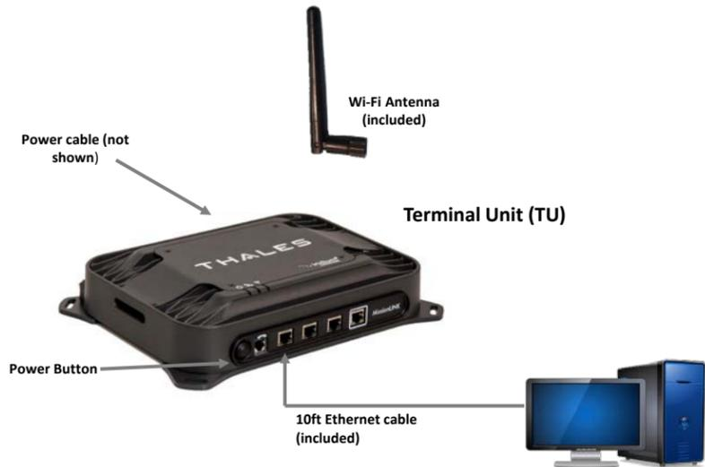
1. Open outer carton, remove Terminal Unit (TU), DC Power Cable, and Ethernet Cable (or Wi-Fi antenna).
