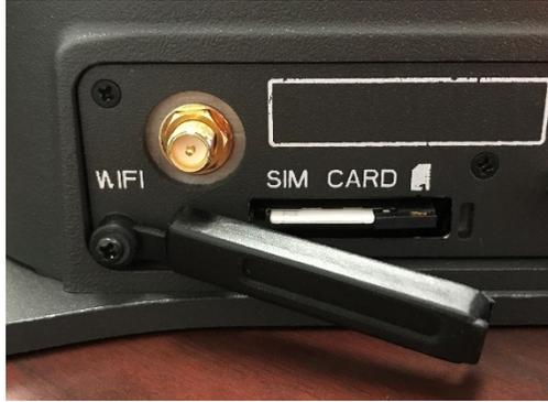
*Figure 2-4 SIM Card with Cover Opened*
