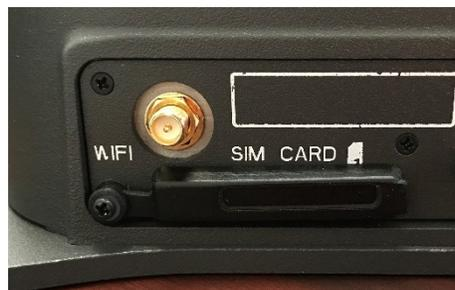
*Figure 2-6 Secure the SIM Card Cover*
