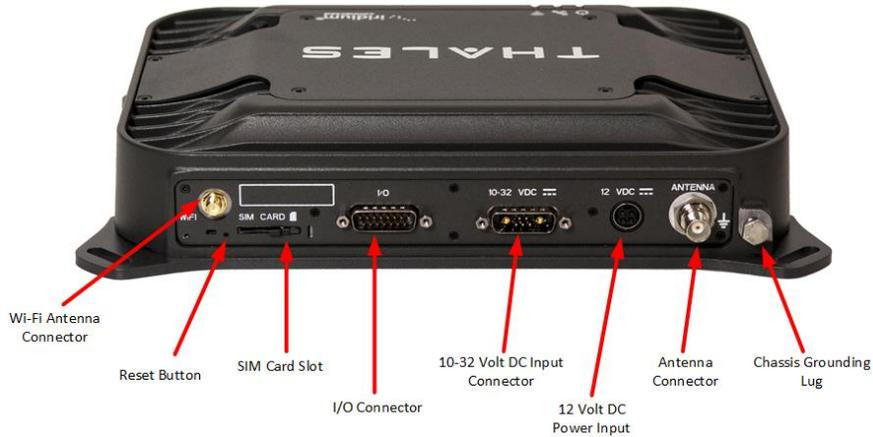
*Figure 1-5 Terminal Unit (TU) Back Panel Detail*
