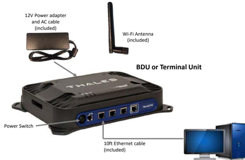
1. Open outer carton, remove BDU, AC adapter, AC Power and Ethernet Cables (or Wi-Fi antenna).
