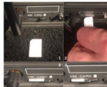
Installing SIM card and engaging the lock
