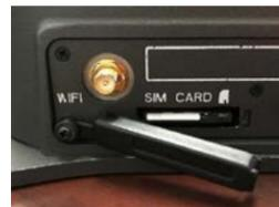
Install SIM card from Air-time provider as below. Insert card with contacts down as shown until it clicks into place. Be sure to engage the lock for the SIM Card and secure the SIM Cover once the SIM Card has been locked into place.
