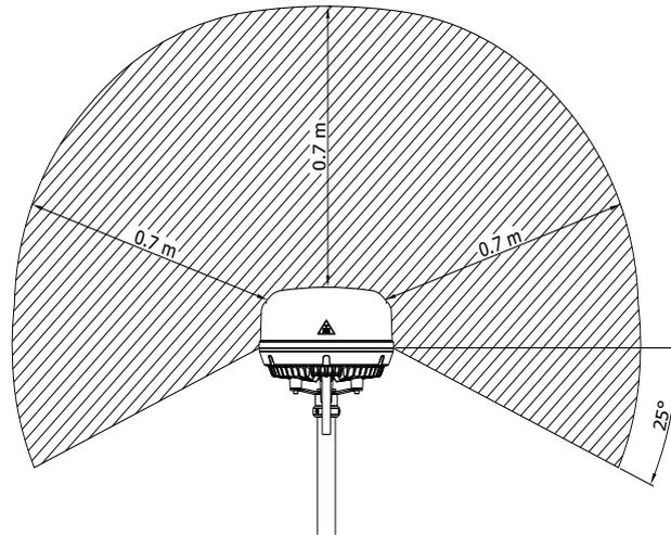
Figure 3-1: Radiation hazard, safety distance
