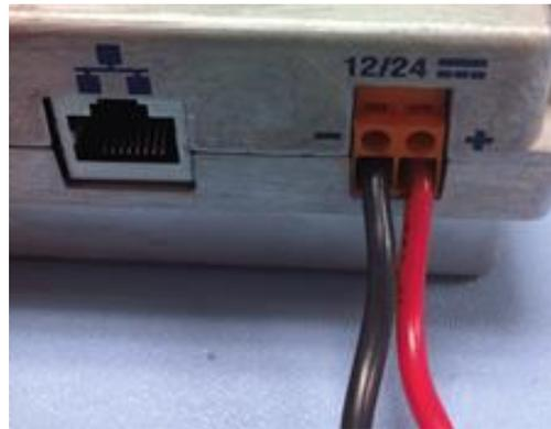
Figure 4-7 - Connecting power leads
