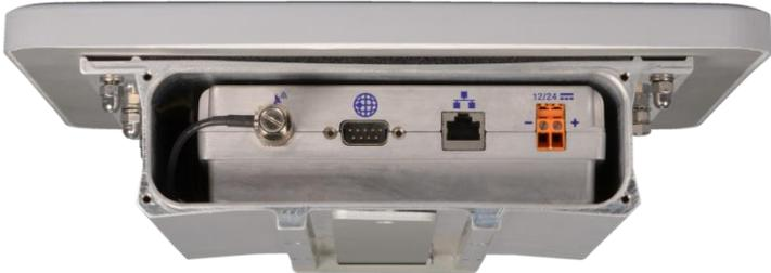
Figure 1-8 - Bottom view with end cap off
