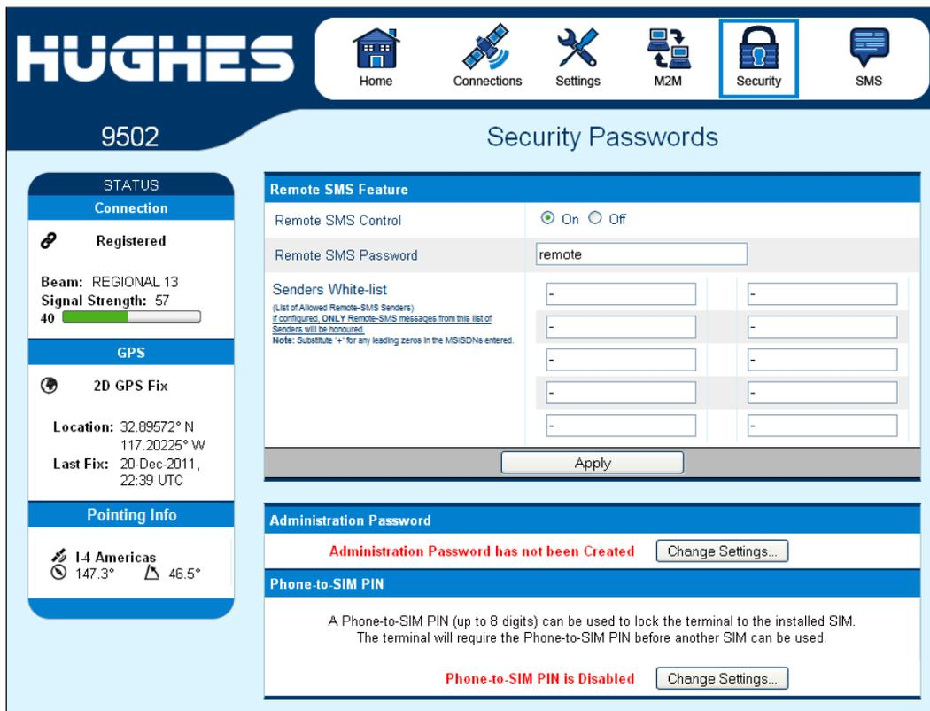
The screenshot displays the 'Security Passwords' configuration page for a Hughes 9502 terminal. The interface includes a top navigation bar with icons for Home, Connections, Settings, M2M, Security (highlighted), and SMS. The main content area is divided into several sections:
