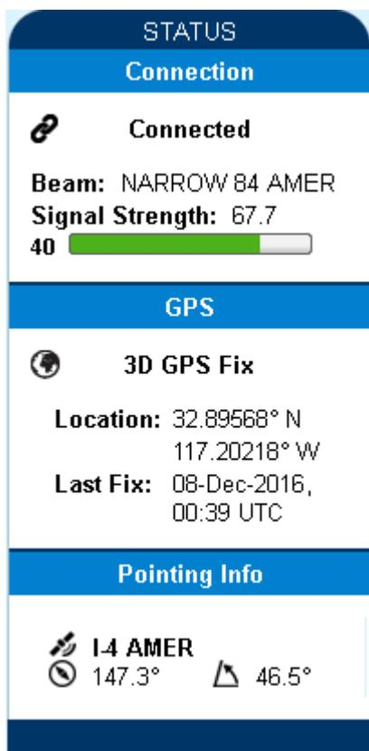
The status bar is included on the home page and other pages that do not have a navigation bar. It includes a field with the elevation angle and compass direction towards the visible satellite(s).
