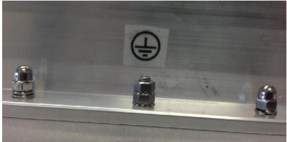
Figure 5-1 – 9502 Protective Earth Grounding
